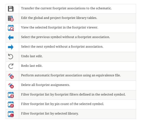
The following table lists the keyboard commands for the Footprint Assignment Tool:
